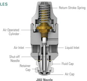
JAU air atomizing nozzles mix compressed air and liquid to form a finely atomized spray. An air-actuated internal cylinder with a return stroke spring cycles the nozzle up to 180 times per minute.
