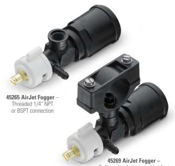
Split-eyelet design provides fast installation of the nozzle onto the liquid supply pipe. No additional pipe fittings are required. Pipe cutting, threading and brazing are eliminated.
