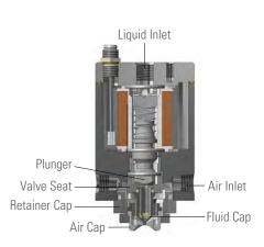
**ELECTRICALLY-ACTUATED AIR ATOMIZING NOZZLES**
